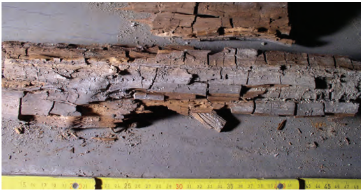
FIGURE 13.1. Brown rot caused by Serpula lacrymans .
